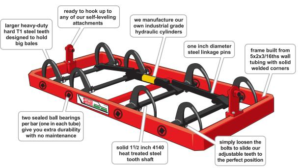
Steffen Systems Bale Handlers are the toughest, longest lasting units available. Their unique opposing spring steel teeth work like a claw, having the strength to curve deep into your tightest bales, yet easily gripping even your softest hay. The sealed ball bearing tooth shaft pivots, and an all steel tubing frame makes the entire unit virtually indestructible. Our Handlers quickly mount to a variety of loaders, and require only one hydraulic remote to operate the teeth.
